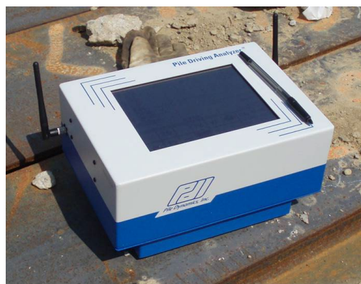
Figure 6. PDA Data Collector
