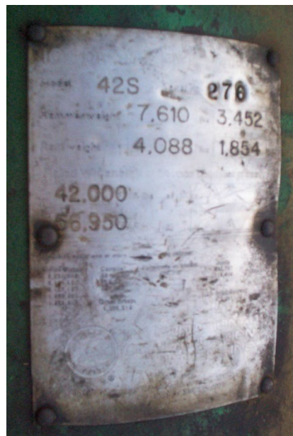
Figure 4. Pile Hammer Data Plate
