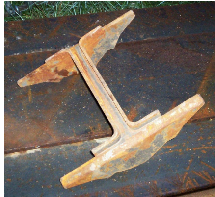
Figure 10. Top (Connection Side) of H-Pile Shoe Tip
