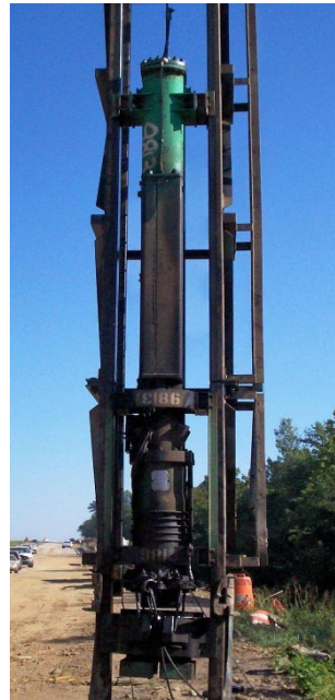
Figure 3. Photo of a Single Acting Diesel Hammer
